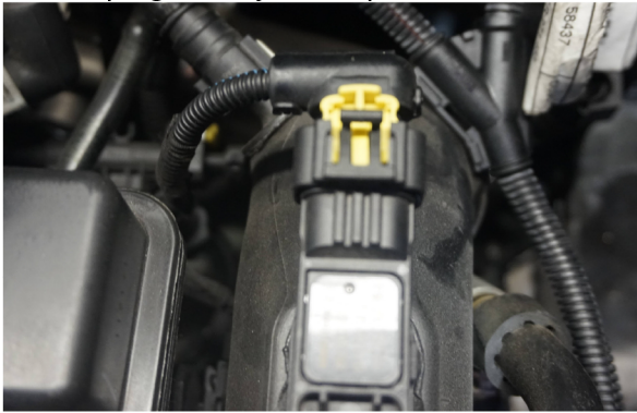
Unplug factory boost pressure sensor
