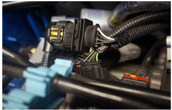
Connect MAP sensor from MAXPower harness
